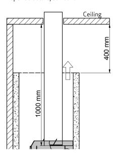
If you want to build in the insert so that the surround is flush with the insert's door, it may be necessary - according to the thickness of the material - to make a cut in the material to allow space for the box on the front.
